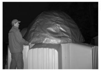
Walk around the POD and pull the cover into place.
